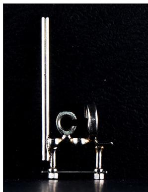
Fig. 2 Torquing key
