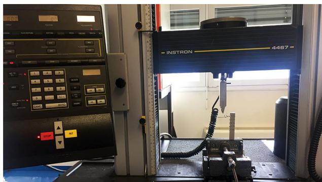
**Fig. 4** INSTRON 4467 dynamometer featuring a 100N load cell and a loading knife
